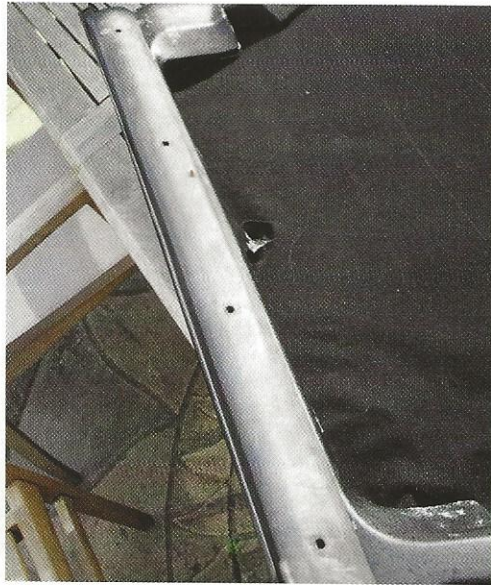
The lateral window seals are fixed to the frame sides and held in place by self-tapping screws accessed through the holes. The steel 'gutter' is still in place
