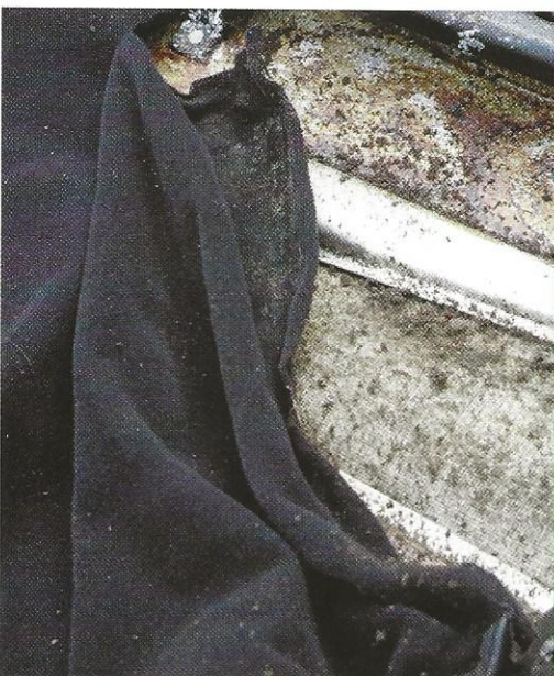
Pulling away the old headlining reveals its poor state, and also the accumulation of dirt and old glue. Note also the poor condition of the roof perimeter frame
