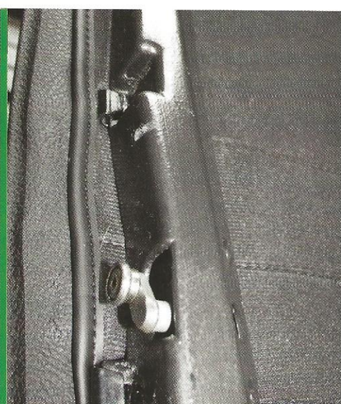
The edges of the leathercloth top and the headlining are held in place by the locating clips. The beading of the headlining is also superglued to make a neat edge
