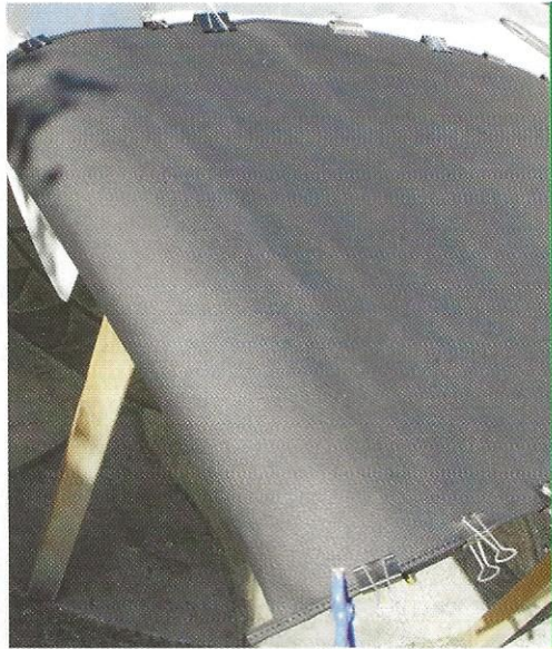
Trial fitting showed just how much stretching of the top (assistant needed) was required. Position of the frame locating clips can be marked on the fold-back...
