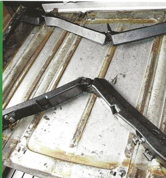
View underside shows the aluminium stiffening plates and the ribs where the headlining is glued. The old linen lining can be seen between the plates
