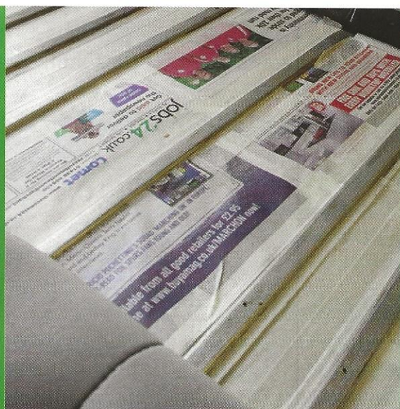
The headlining is glued only to the ribs on the underside of the plates, so the remaining areas need to be masked. As the linen, work slowly to avoid wrinkles
