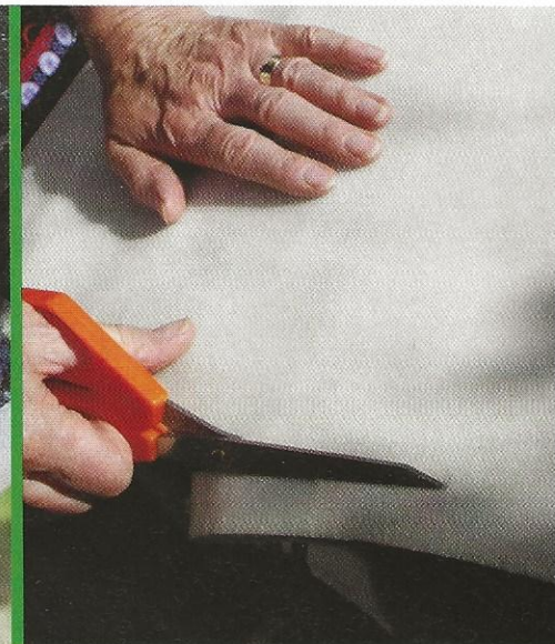
The foam insulation is trimmed fractionally under-size and then stuck to the linen with glue only around the edges to allow flexibility when folding the roof
