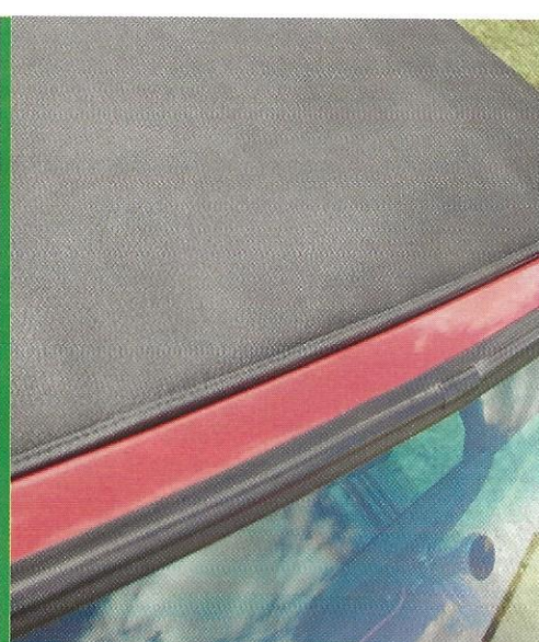
No more patches or cracked edging. It's important to get the beaded edge of the roof covering angled down slightly for a snug fit against the windscreen frame
