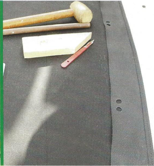
...and with the top off the frame, holes in the leathercloth can be cut for the bolts: wood block underneath, mark with the pipe/mallet, cut out with modelling knife
