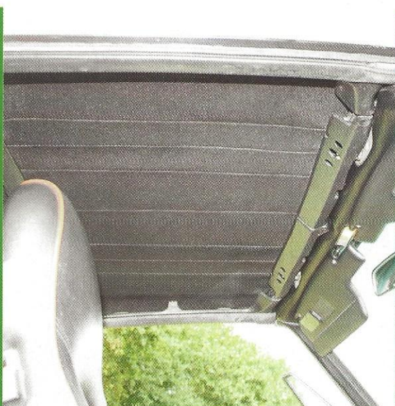
Targa top back where it should be! Note neat fitting headlining and the Hammerite re-painted perimeter frame. Now I'm waiting for rain and a good run to see if it leaks
