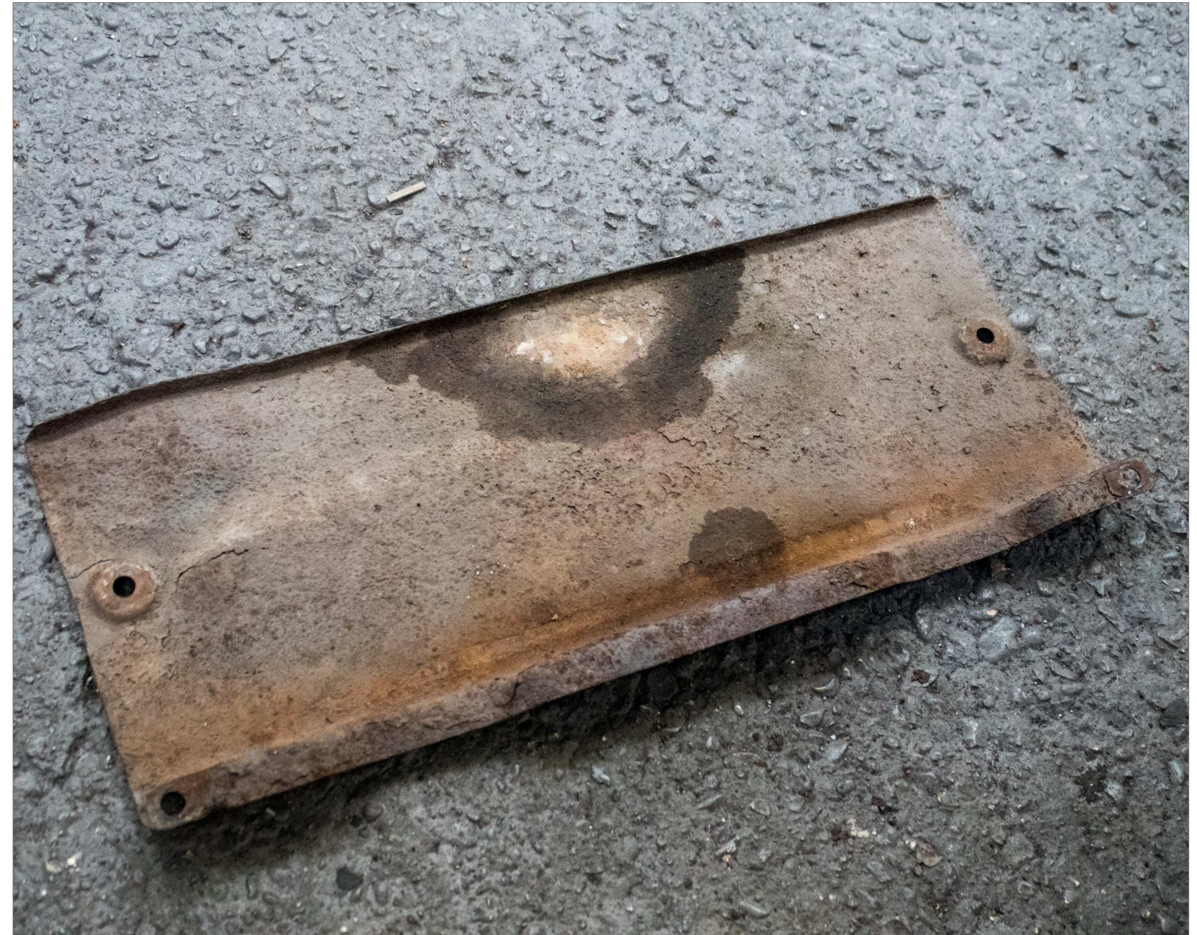
Shown here is the fuel pump cover removed.
