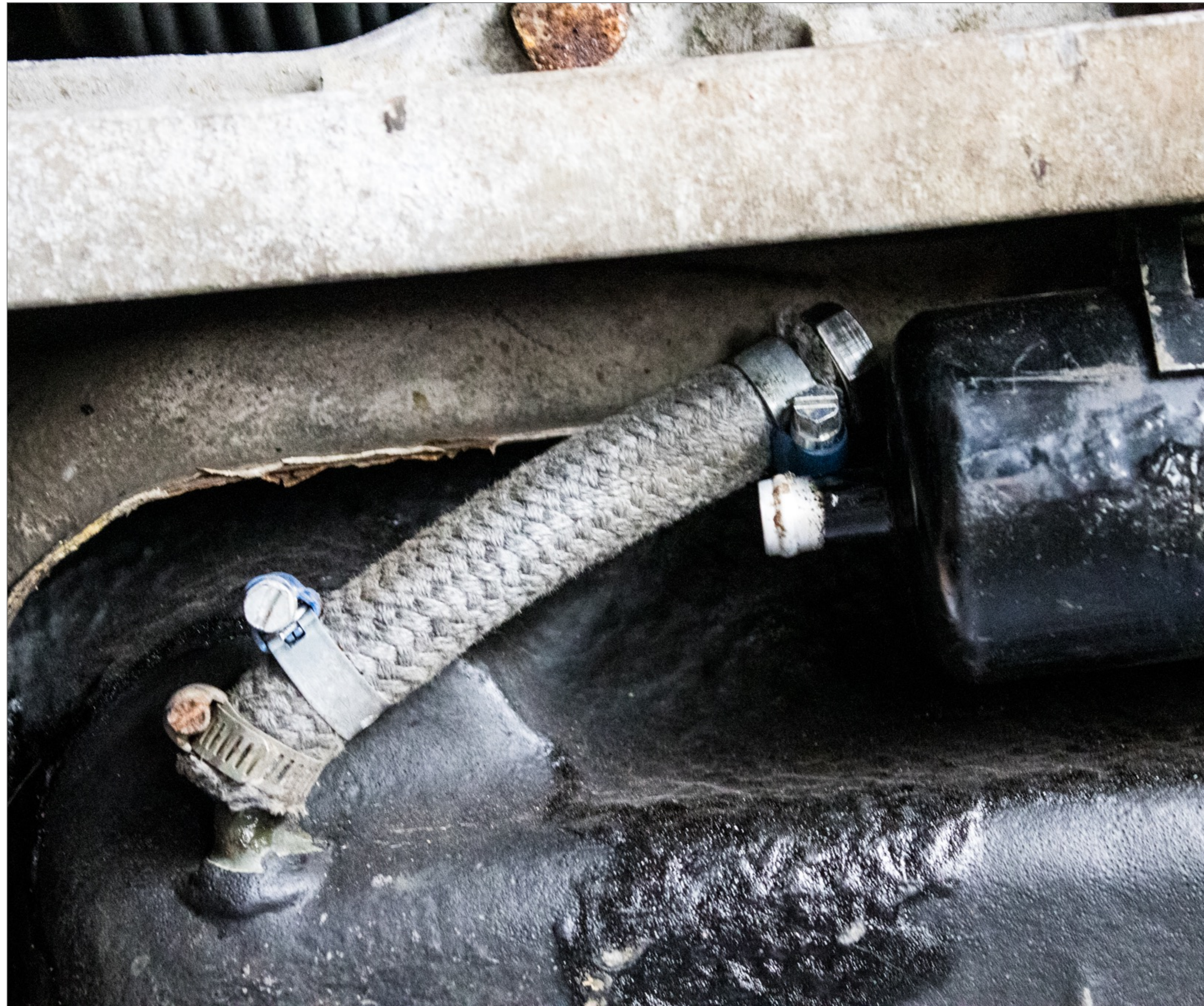
Fuel pipes going to the fuel pump can be removed to drain the tank.
