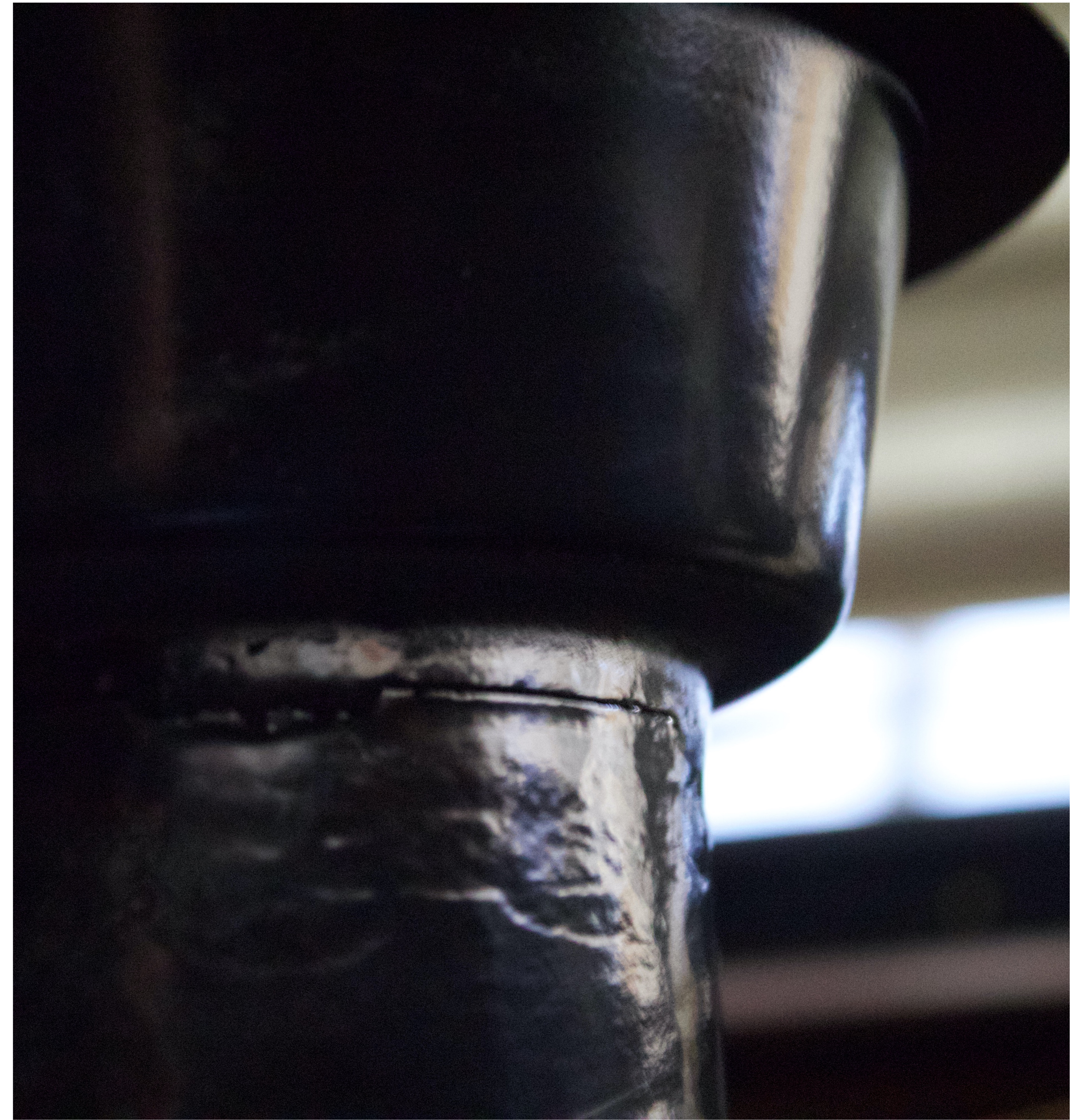
Weld the collar onto the filler neck as per your measurements.
