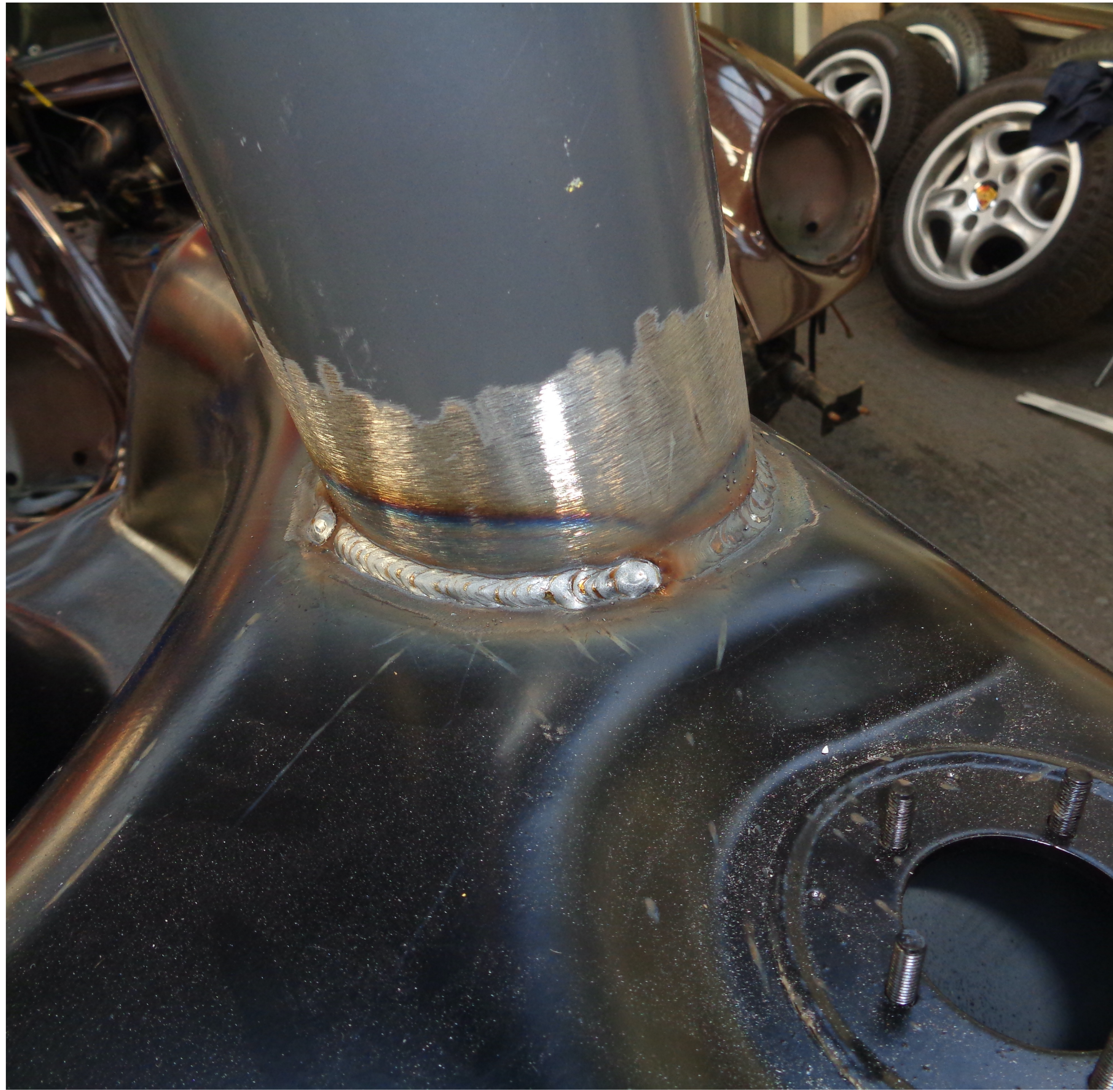
Weld the filler neck into position as per your measurements.
