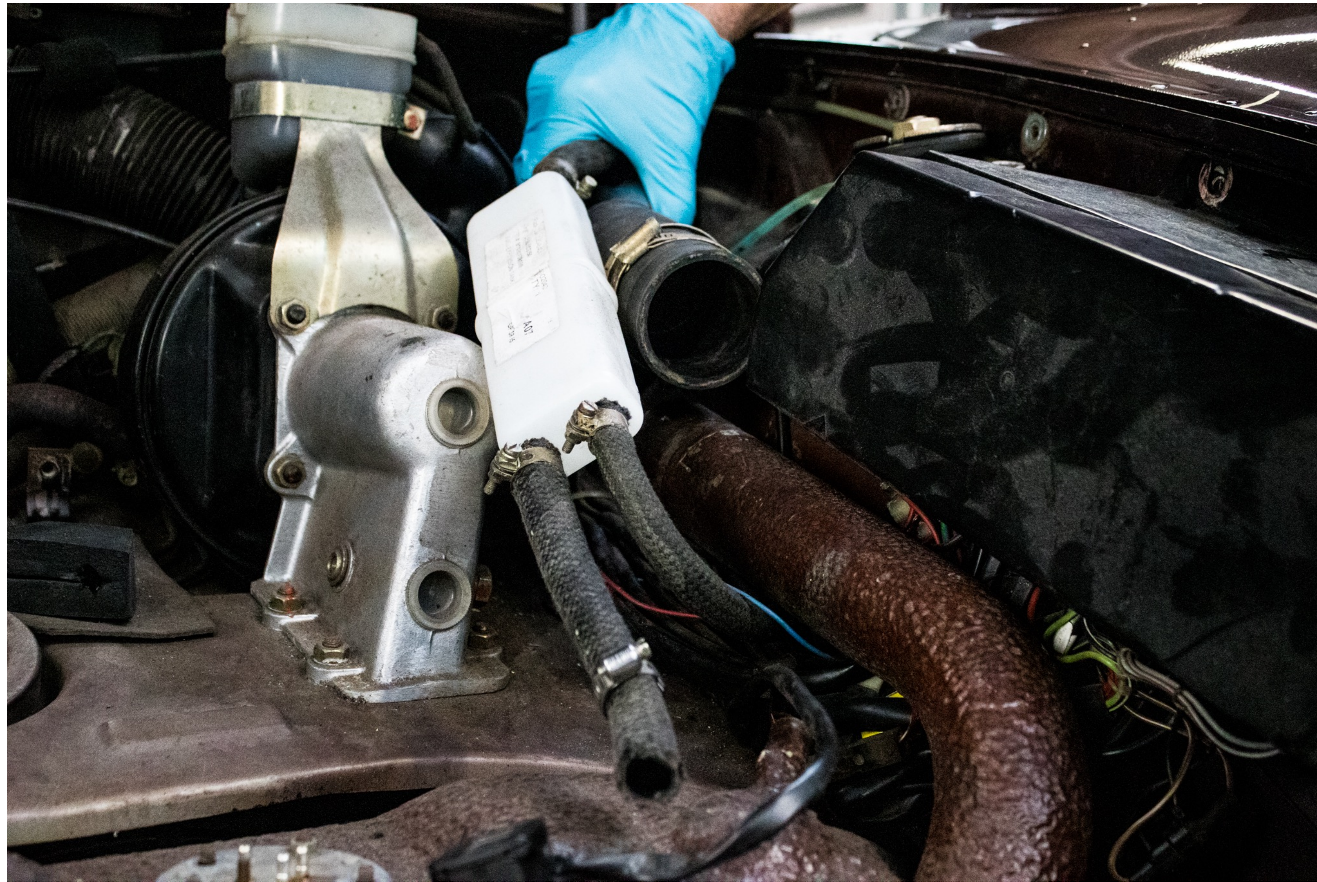
Remove the fuel breather system and filler neck connecting tube. Fuel tank slender unit wiring.
